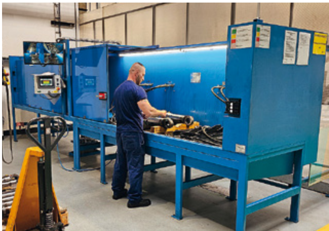
- Pressure, functional and cleanliness test
