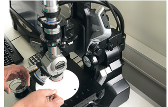
- Microscope + test result according VDA19
