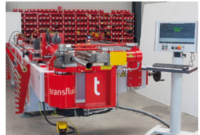
- TRANSFLUID bending machine for tube diameters up to 42 mm
